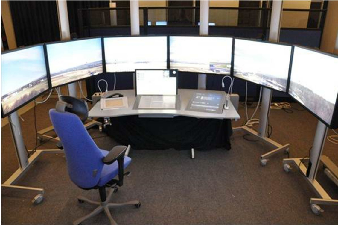
Figure 21 - Remote Tower Test Facility (showing CWP and front 240° screens)
