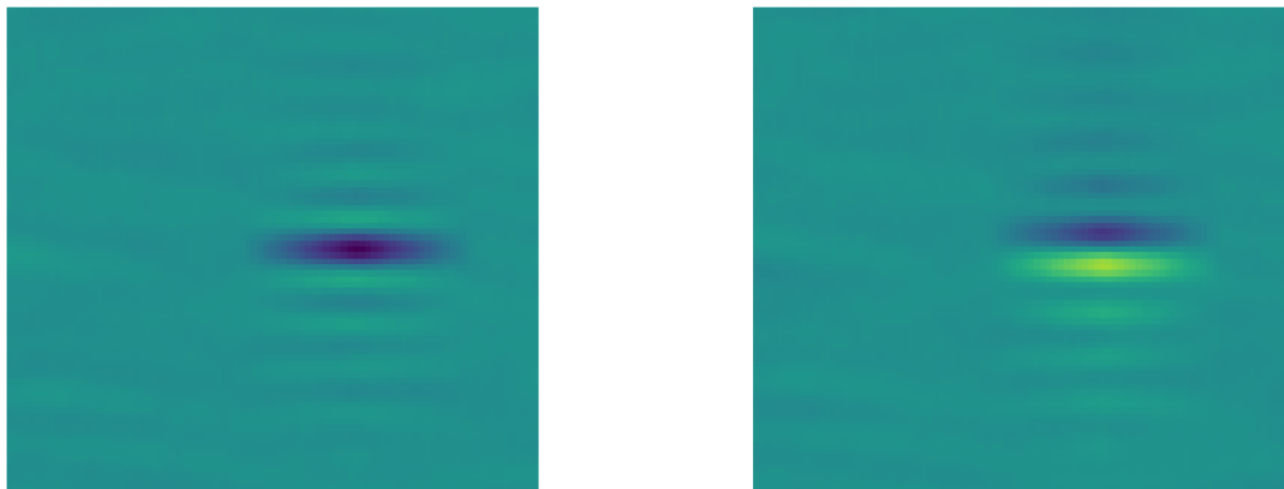
Figure 7: The I and Q correlator outputs of the synthetic data generator as images, PRN number set to 1
